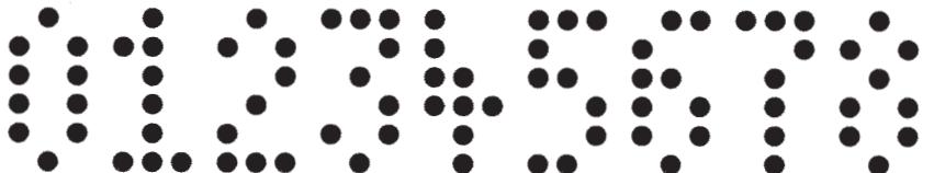
20 mm condensed, matrix 3 x 6, pin Ø 2.3 mm
